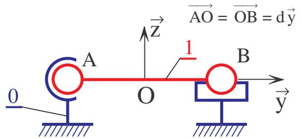
$$\{A0 \rightarrow 1\} = \begin{Bmatrix} X_A & 0 \\ Y_A & 0 \\ Z_A & 0 \end{Bmatrix}_{A, \vec{x}, \vec{y}, \vec{z}} ; \{B0 \rightarrow 1\} = \begin{Bmatrix} X_B & 0 \\ 0 & 0 \\ Z_B & 0 \end{Bmatrix}_{B, \vec{x}, \vec{y}, \vec{z}}$$
