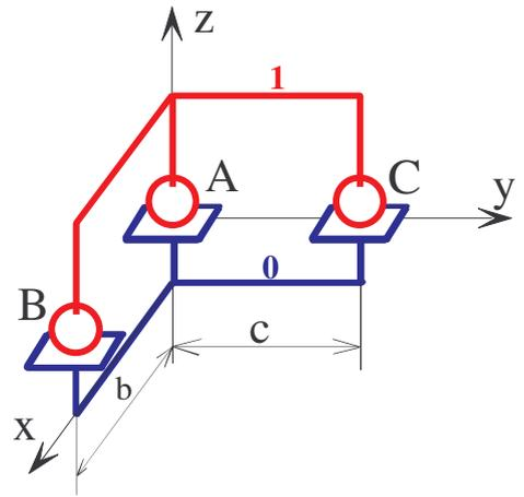
$$\{A0 \rightarrow 1\} = \begin{Bmatrix} Z_A \vec{z} \\ \vec{0} \end{Bmatrix}_A ; \{B0 \rightarrow 1\} = \begin{Bmatrix} Z_B \vec{z} \\ \vec{0} \end{Bmatrix}_B ; \{C0 \rightarrow 1\} = \begin{Bmatrix} Z_C \vec{z} \\ \vec{0} \end{Bmatrix}_C$$
