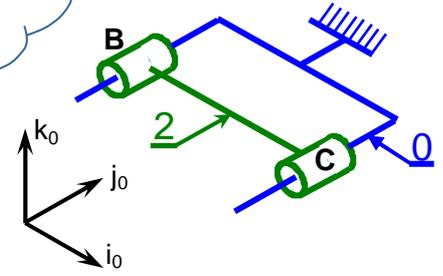
$$\left\{ \mathcal{V}_{L_B}^{2/0} \right\}_B = \begin{Bmatrix} \beta_{B_{2/0}} \cdot \vec{j}_0 \\ \nu_{B_{2/0}} \cdot \vec{j}_0 \end{Bmatrix} \quad \left\{ \mathcal{V}_{L_C}^{2/0} \right\}_C = \begin{Bmatrix} \beta_{C_{2/0}} \cdot \vec{j}_0 \\ \nu_{C_{2/0}} \cdot \vec{j}_0 \end{Bmatrix}$$
