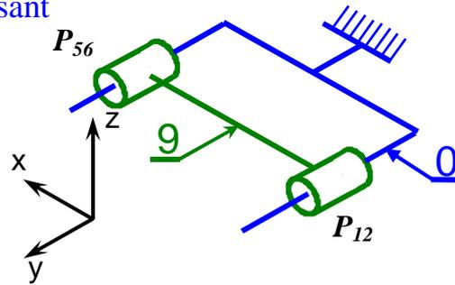
$$\begin{aligned} \overline{V(P_{12}, 9/0)}_{(L_{5678})} &= \overline{V(P_{56}, 9/0)}_{(L_{5678})} + P_{12}P_{56} \wedge \overline{\Omega_{9/0}}_{(L_{5678})} \\ &= v_{5678,9/0} \cdot \vec{y} + L \cdot \vec{x} \wedge \beta_{5678,9/0} \cdot \vec{y} = v_{5678,9/0} \cdot \vec{y} + L \cdot \beta_{5678,9/0} \cdot \vec{z} \end{aligned}$$
