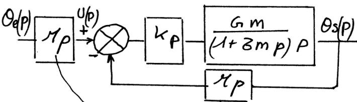
3324 - Calculer la fonction de transfert  $H_g(p) = \frac{\Theta_s(p)}{\Theta_e(p)} = \frac{k_p G_m \gamma_p}{k_p G_m \gamma_p + p + \beta_m p^2}$ .
