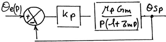
$$H_g(p) = \frac{1}{1 + \frac{p}{k_p G_m \gamma_p} + \frac{\beta_m}{k_p G_m \gamma_p} p^2}$$
